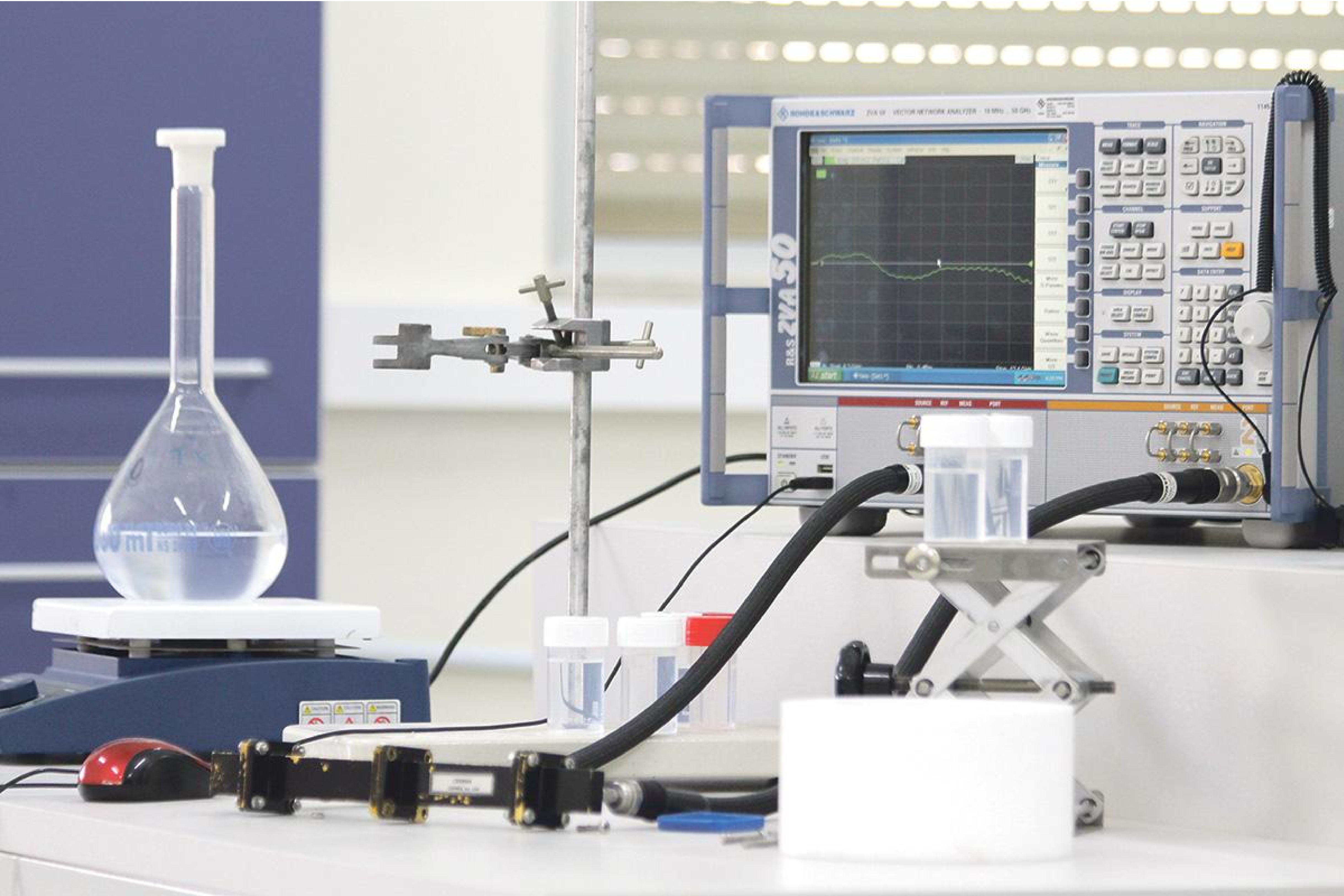
The Vector Network Analyser (VNA) that is currently housed at the University of Malta. This VNA is normally used to perform reflection measurements on biological samples to measure the dielectric properties. Photo: Julian Bonello
